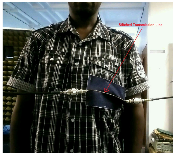
Figure 6. ON BODY measurements on the stitched transmission line [19]
