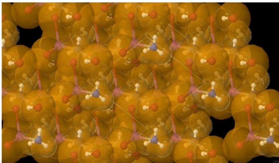
Figure 4. JMOL Render of  $\text{CH}_3\text{NH}_3\text{BiBr}_3$  BCC crystal structure showing localized molecular
